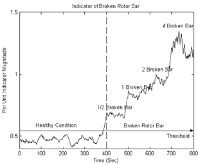
Fig. 11. Indicator of Broken Rotor Bar
