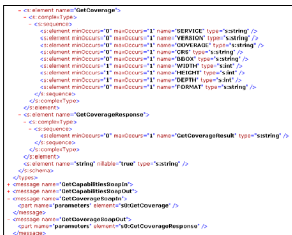
Fig. 4. This figure shows a part of WSDL documents: details on a GetCoverage operation
